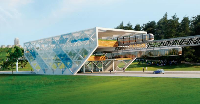
A lightweight pre-stressed overpass with thin composite rails without expansion joints throughout the whole length is used as a track. Passengers and cargo are transported by steel-wheeled electric vehicles equipped with an automatic control system.
