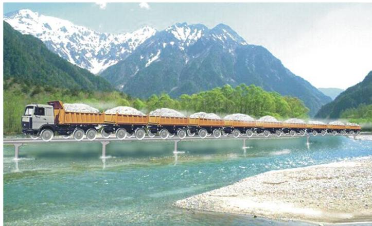
Fig. 10. Freight STU train (megaSTU) for carrying friable freights in mountainous conditions
