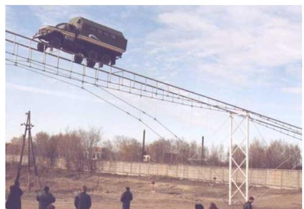
Fig. 42. Modified ZIL-131 on a 48 m string span (November, 2003)
