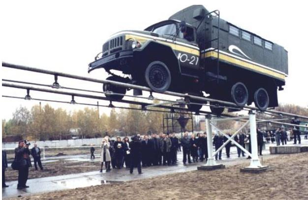
Fig. 41. Modified ZIL-131 on a 24 m string span (October, 2001)
