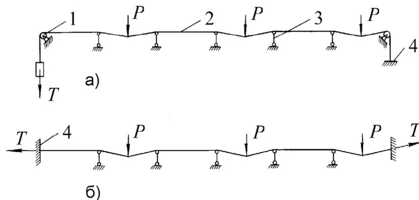
Fig. 17. String linear scheme: a) with a block at the end of a string; b) with a string sealed off;
