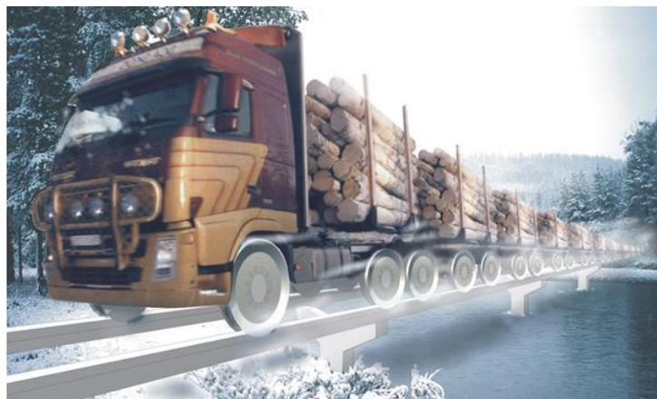
Fig. 12. Freight STU train (megaSTU) for carrying timber
