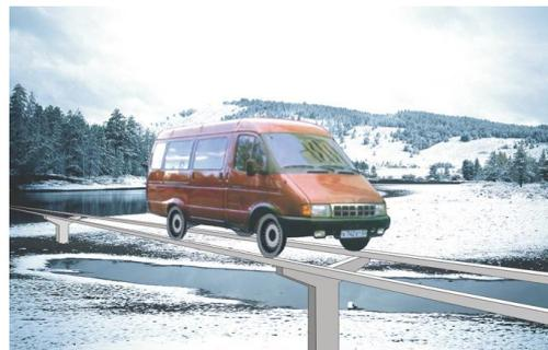
Fig. 6. Mini-bus on string-rails
