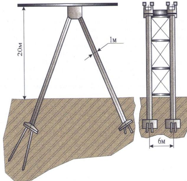
Fig. 19. Anchor support of a double-track STU route
