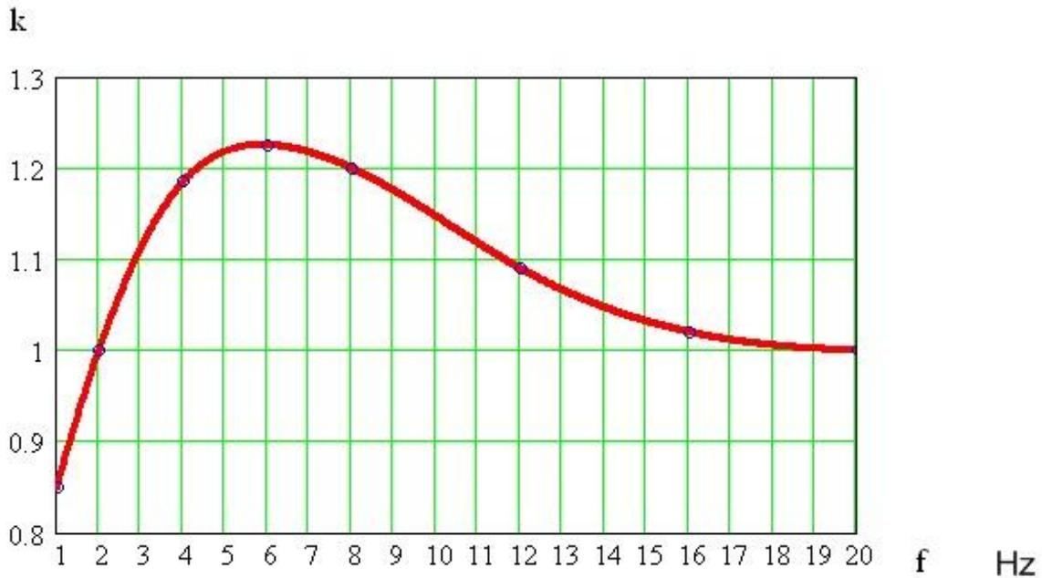
Fig. 2.69. Dependency of k coefficient on the frequency of vertical oscillations
