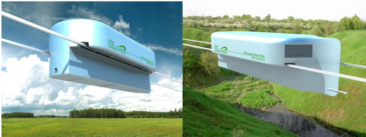
Fig. 3.43. General view of suspended STS (on the left there is front view of a unicar; on the right there is rear view of a unicar)
