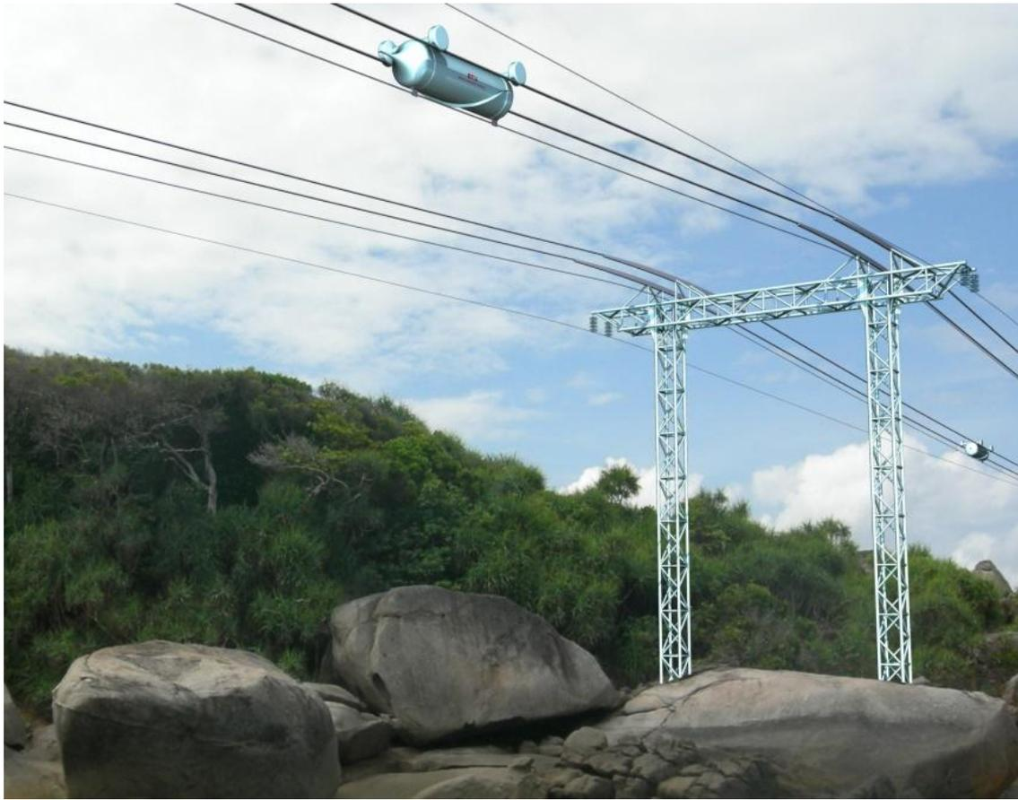
Fig. 1.1. Traction rope version of freight suspended STU
