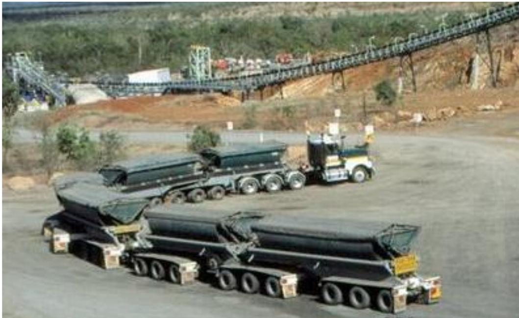
Fig. 3.11. “Road trains” are widely used in Australia in mining transportation
