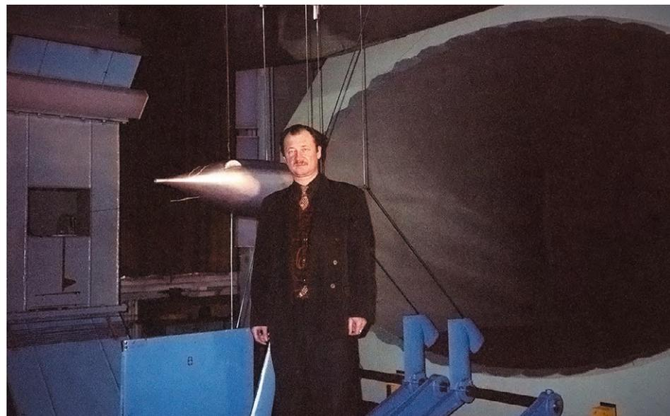
Wind-tunnel test of a high-speed unibus model (scale 1 : 5).
