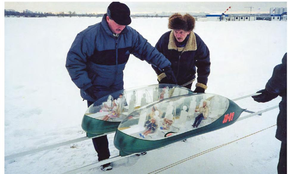
First test of a double-rail track and a double-body unibus model (scale 1 : 5).
