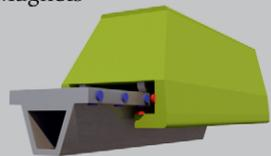
The track structure operation is more labour intensive due to its complicated configuration and technical components (electric coils, switching devices, etc.), which require constant maintenance and machinery for cleaning the track from snow and icing.
