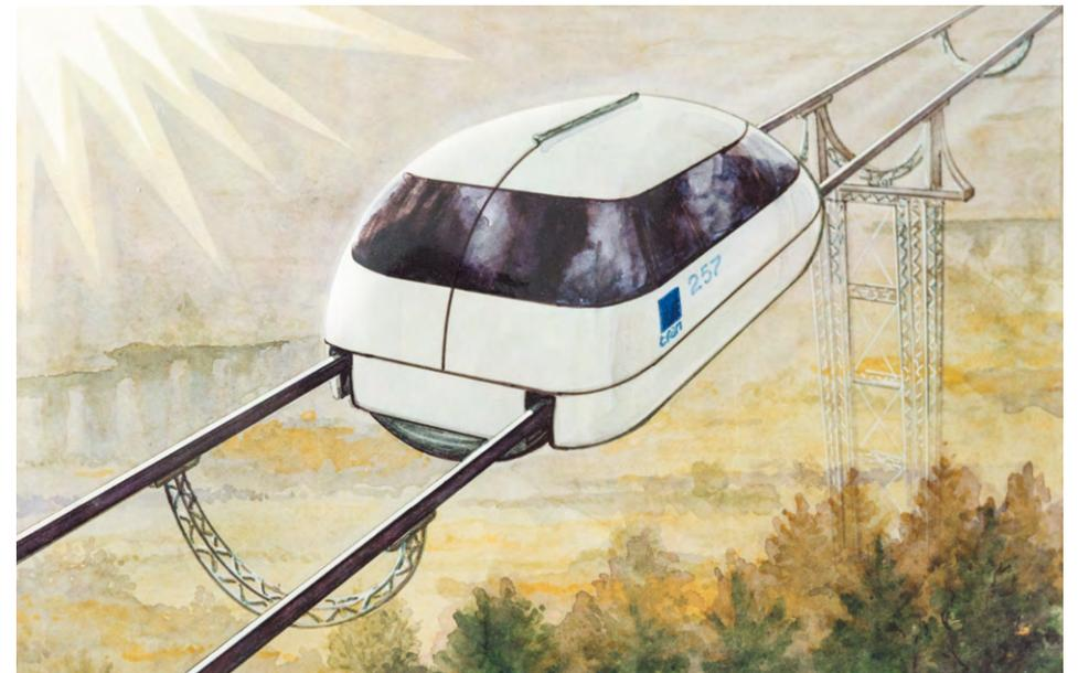
Figure 1.5 – NTL track on tower supports (about 100 m)
