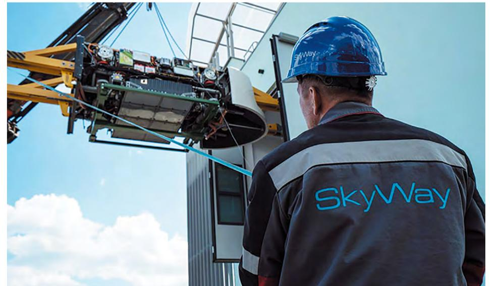
Testing of traction modules of a double-rail unibus UR-220.
