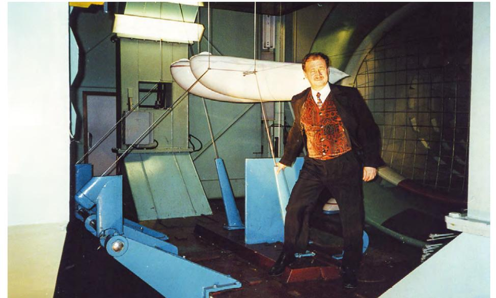
Wind-tunnel test of a double-body unibus model (scale 1 : 5).
