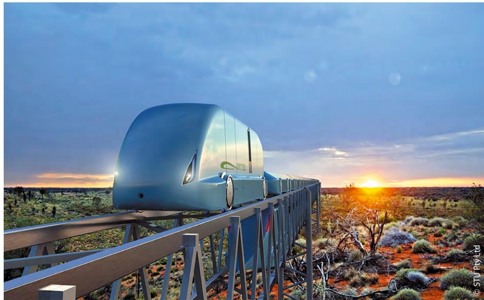
SkyWay cargo mounted train on a double-track string truss-type overpass (visualization). 2011
