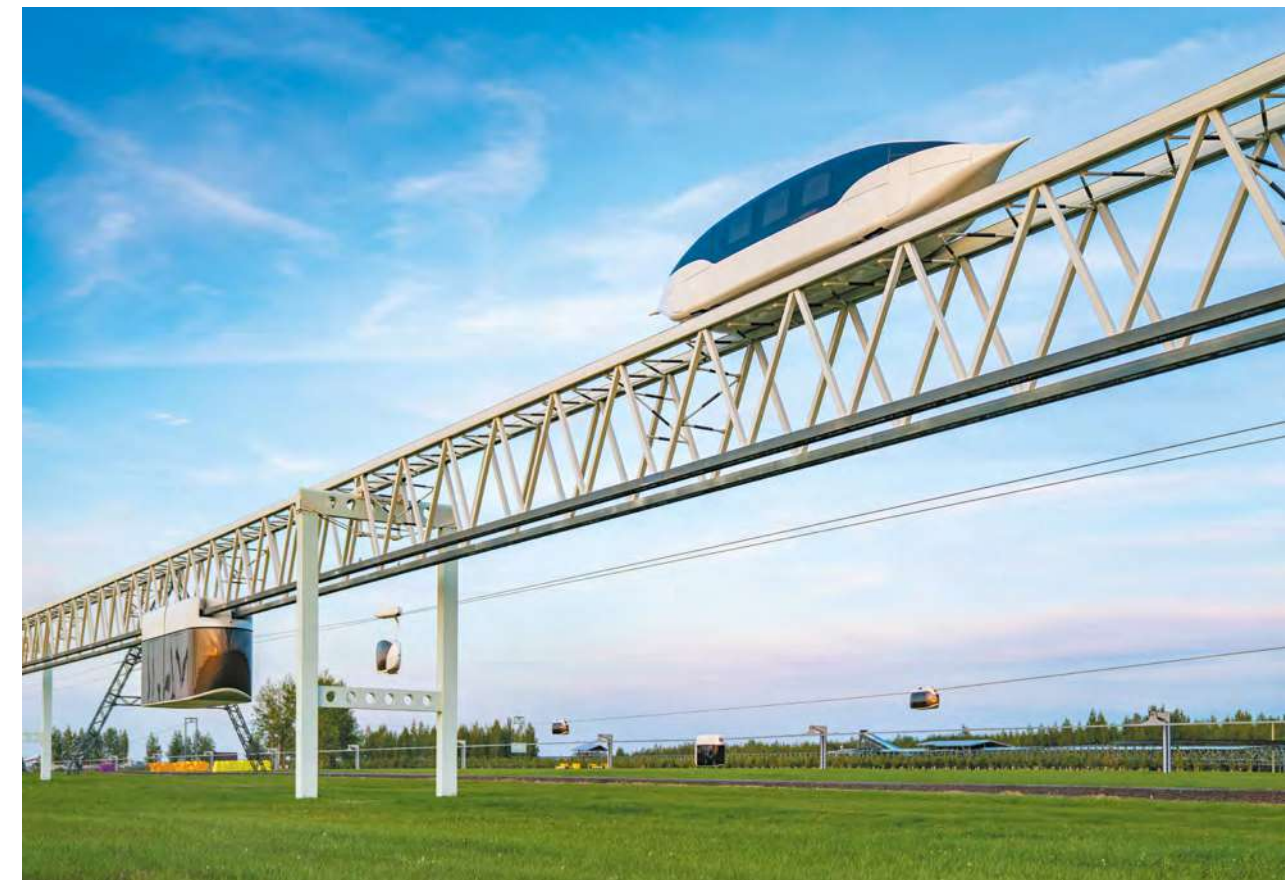
2019. EcoTechnoPark. Different types of string transport rolling stock – six uPods (including high-speed transport module) – on various types of string overpasses
