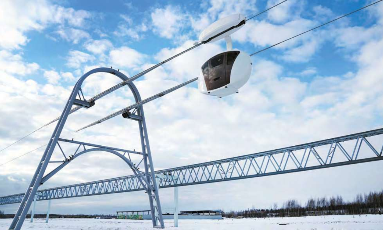
2019. EcoTechnoPark. uWind – one of the simplest models in the range of string transport rolling stock. Cargo uTruck designed for transportation of bulk cargo
