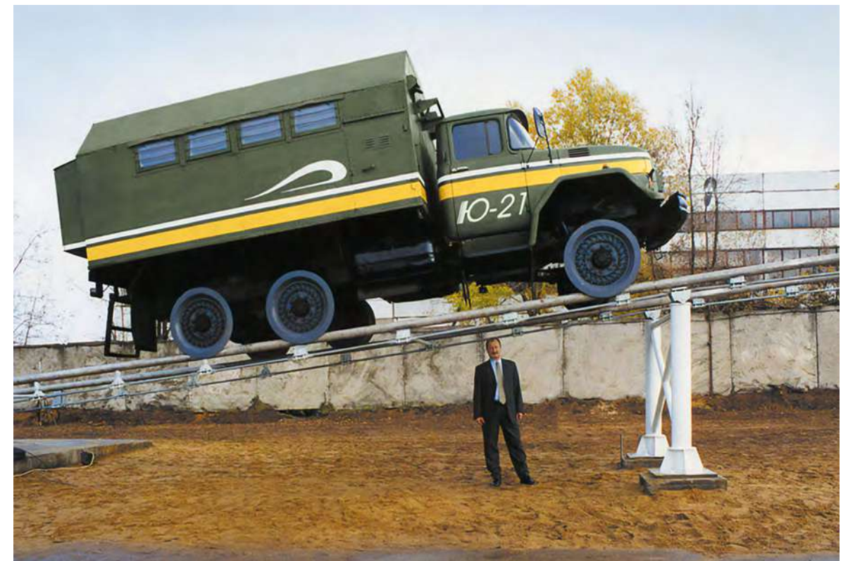
2001. Testing the string transport at the Ozyory test site. I demonstrated the reliability and safety of the system, while standing under the track structure along which the rolling stock simulator based on the ZIL-131 truck with a weight of over 10 tons was moving
