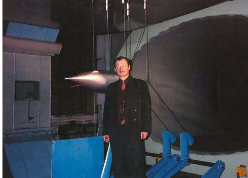
1996. City of St. Petersburg. Air blowdown of 1 : 5 scale model of high-speed module in airflow test tube
