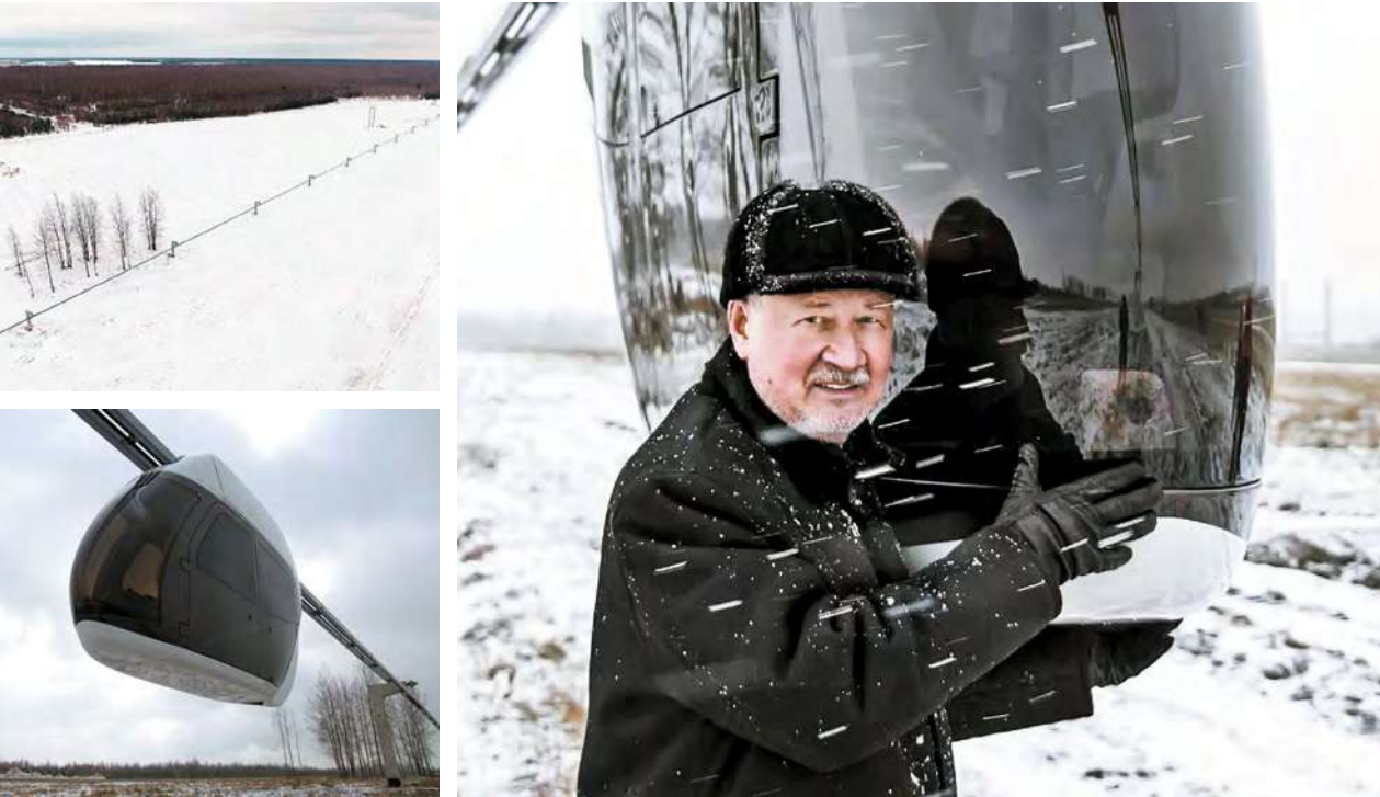
2016. EcoTechnoPark. Stretching the string rail and start of running tests of light transport system and two-seat string vehicle
