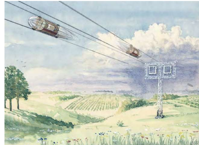
String transport and string-rail overpass – a type of transport systems developed by Anatoli Unitsky, in which transportation of passengers and cargo is carried out on special overpasses consisting of string rails, supporting towers, and anchoring structures. The rails have prestressed wires or steel ropes (strings) inside. The string-rail overpass has unique features, provides significant material savings in the construction of communications and allows to increase speed, comfort, and safety of traffic. A variety of electric vehicles on steel wheels is used as rolling stock. The systems control is fully automated.
